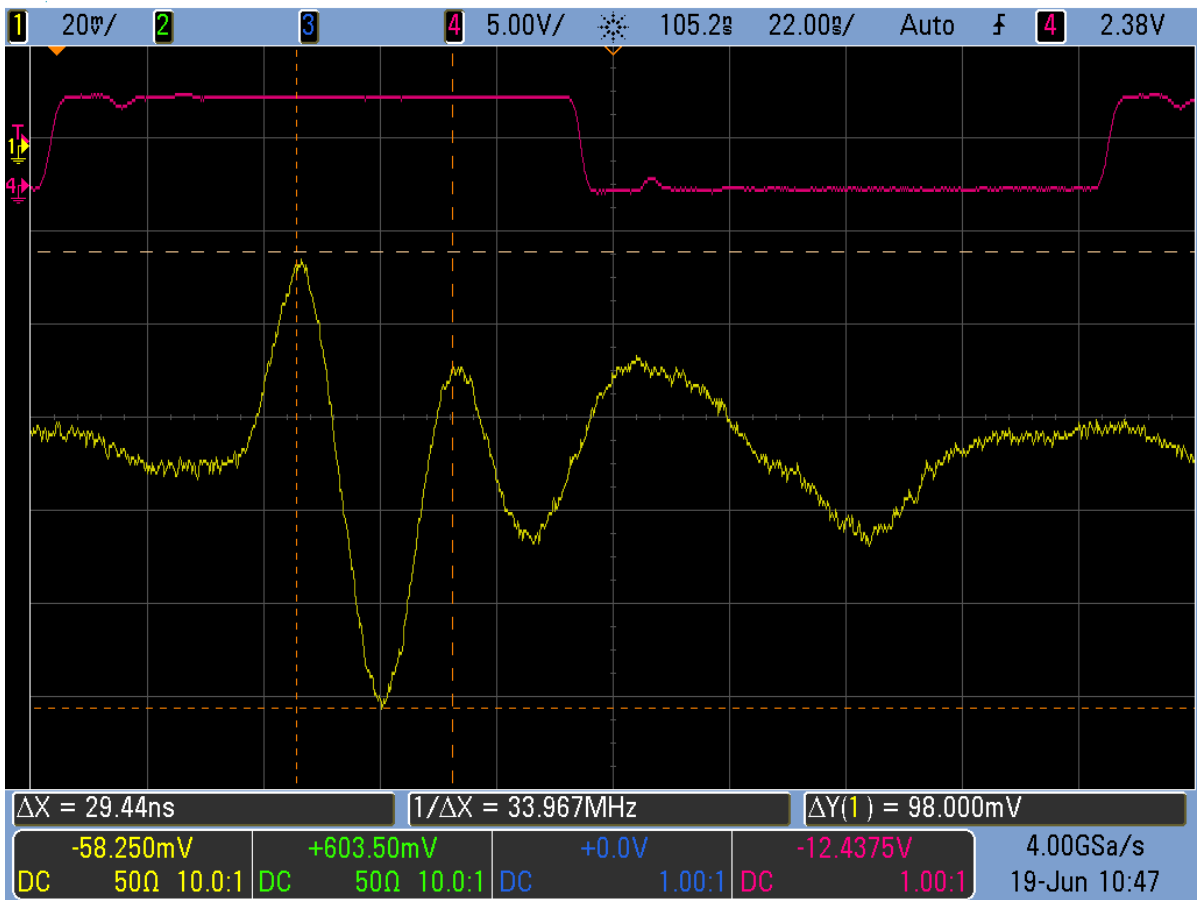
Figure 286: B1A4, S2D response at 5 MHz of main clock. Input pads not bonded.
