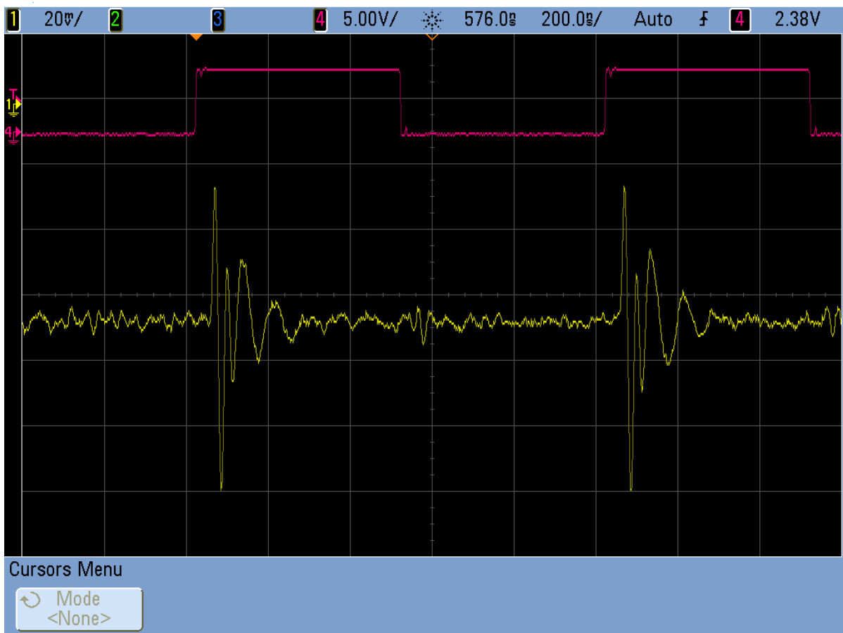
Figure 276: B1A4, S2D response at 1 MHz of main clock. Rising edge corresponds to the ADC conversion. Input pads not bonded.
