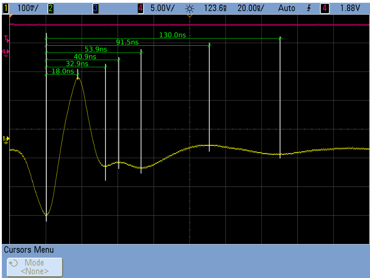
Figure 284: B1A4, Time structure of S2D response at 1 MHz. 12 pF at inputs. Preamp GND – input + backside
