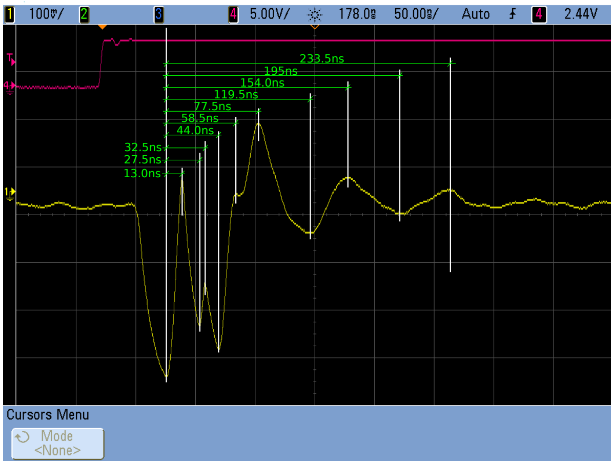
Figure 81: B1A4, Time structure of S2D response at 1 MHz. 12 pF at inputs.
