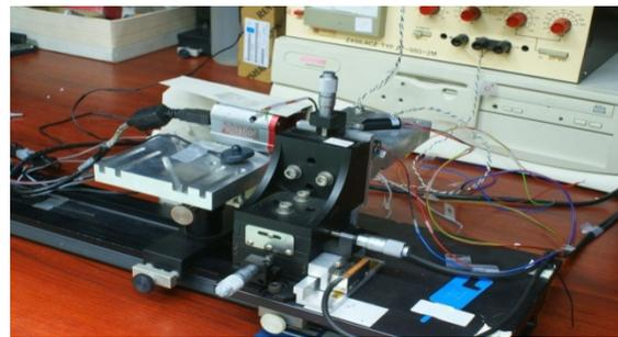
Figure 4. Picture of the new laboratory setup with CCD camera, Renishaw RG24 optical heads and two laser beams.
