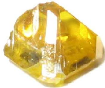
**Figure 1. Typical diamond crystal synthesized with temperature gradient method at "Adamas" plant.**
