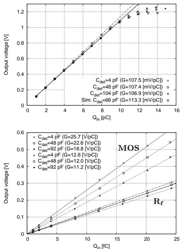
Fig. 6. Gain measured in physics mode for channels with MOS feedback (upper), in calibration mode (lower) for channels with MOS and passive  $R_f$  feedback
