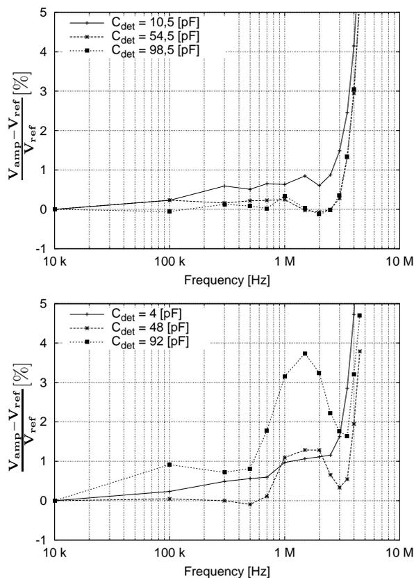
Fig. 8. Amplitude change for  $R_f$  resistor front-end channels in physics mode (upper) and in calibration mode (lower)
