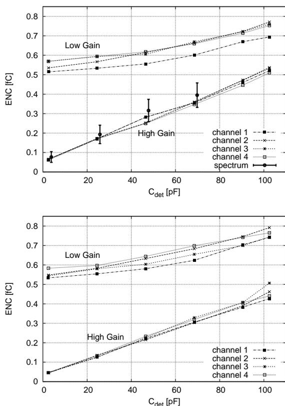
Fig. 7. Noise ENC measurements obtained with true RMS meter for the front-end with passive feedback (upper) and active feedback (lower)
