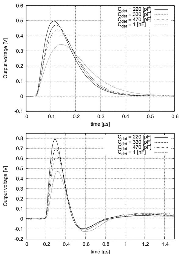
Fig. 5. Output pulses for MOS feedback channels in physics mode (upper) and in calibration mode (lower) for extremely large input capacitances. In calibration mode  $Q_{in} = 40$  fC, while in physics mode  $Q_{in} = 4.95$  pC
