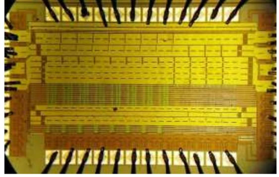
Fig. 3. Photograph of glued and bonded prototype. First 4 channels from the left have passive feedback and next 4 channels have active feedback
