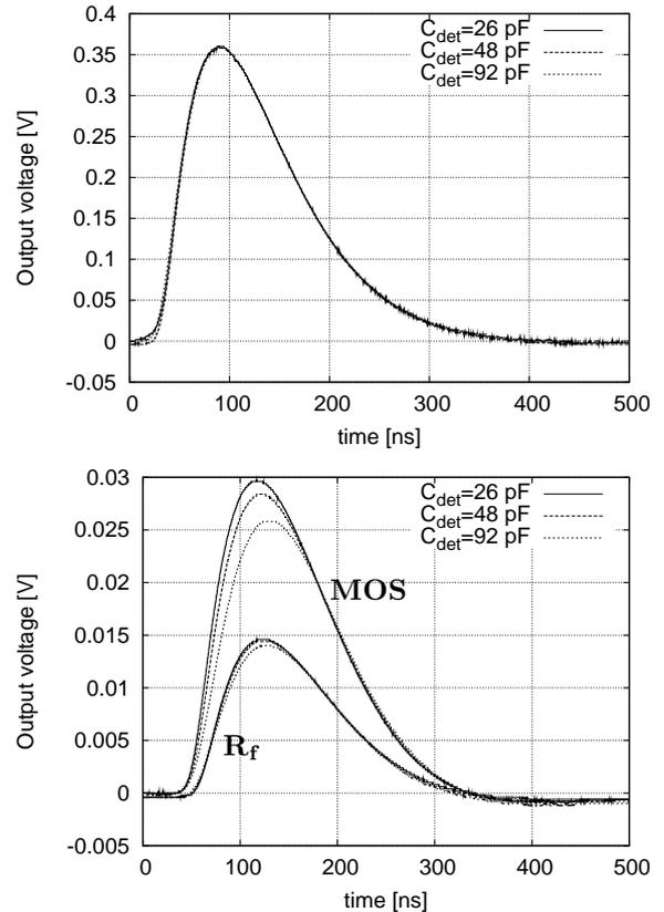
Fig. 4. Output pulses for MOS resistor front-end channels in physics mode (upper) and for MOS and  $R_f$  resistor in calibration mode (lower), as a function of input capacitance. In calibration mode  $Q_{in} = 10$  fC, while in physics mode  $Q_{in} = 3.3$  pC
