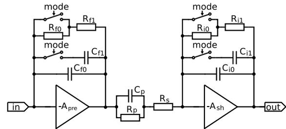
Fig. 1. Block diagram of a single front-end channel
