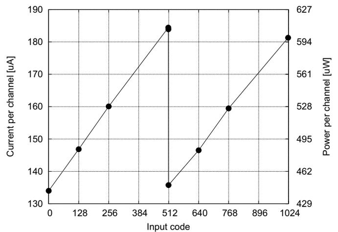
Fig. 10. Power consumptions vs DAC input code.
