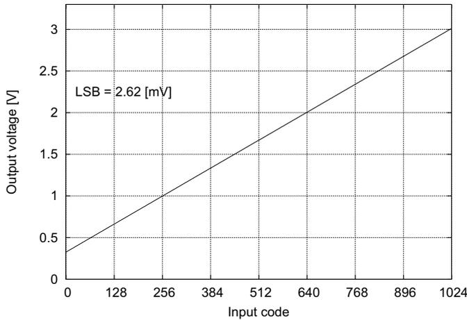
Fig. 6. Output voltage vs DAC input code.
