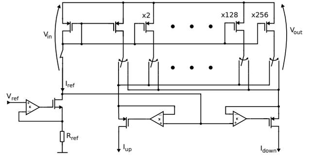
Fig. 2. Block diagram of active cascode stage.
