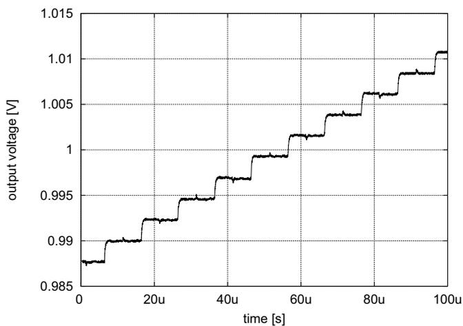
Fig. 9. Waveform showing 1 LSB steps transient
