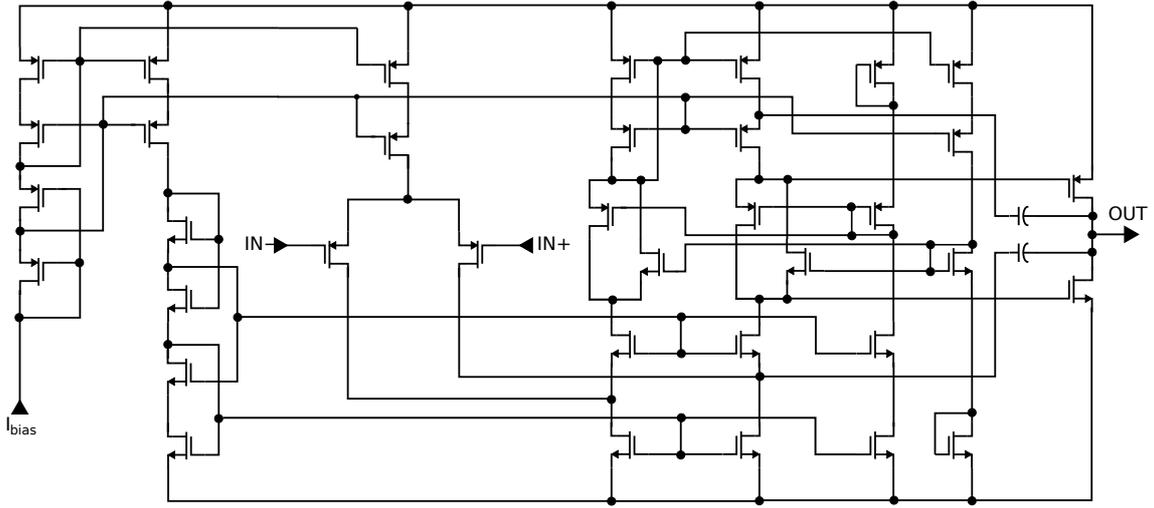
Fig. 4. Schematic diagram of class AB output amplifier.
