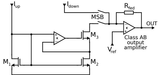
Fig. 3. Block diagram of high swing output circuit.
