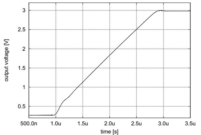
Fig. 8. Waveform showing settling between 0 and 1023 input code
