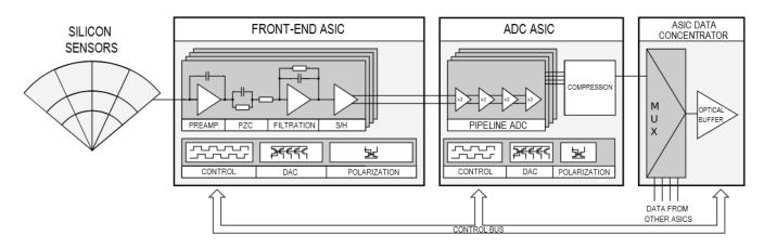
Figure 1.5: LumiCal's readout electronics flow chart. Reproduced from [10].
