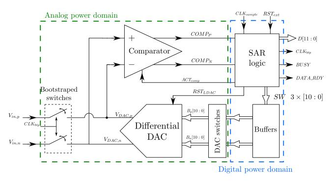
Figure 4.1: Block schematic of designed 12-bit SAR ADC.
