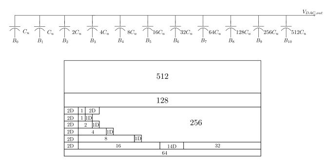
Figure 4.6: Schematics and layout floor-plan for MOM-capacitor based DAC (capacitor sizes are not to scale). Letter D indicates dummy capacitors.
