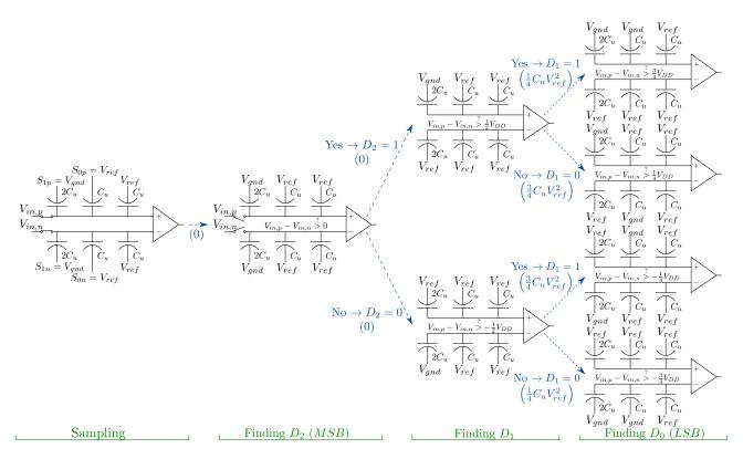
Figure 3.23: 3-bit SAR ADC incorporating switchback switching algorithm.
