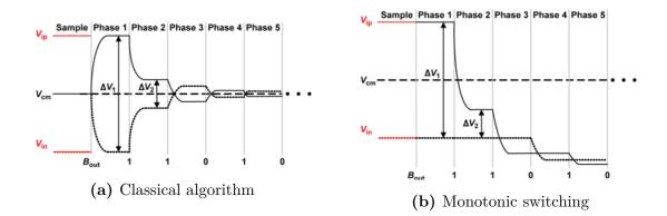
Figure 3.6: Comparison of voltage on DACs top plates during conversion using classical algorithm and monotonic switching. [19]
