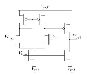
Figure 3.43: Two-stage open loop comparator [37]
