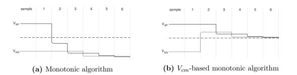
Figure 3.28: Comparison of voltage on DACs top plates during conversion using monotonic and  $V_{cm}$ -based monotonic algorithms. [29]
