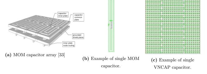
Figure 4.5: Examples of MOM and VNCAP capacitors (not to scale).
