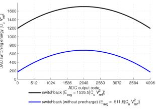
Figure 3.22: Energy consumption due to DAC switching for 12-bit ADC using switchback algorithm.
