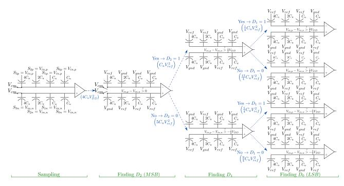
Figure 3.2: 3-bit SAR ADC incorporating classical algorithm.
