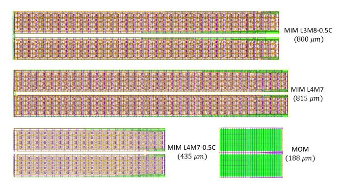
Figure 4.9: comparison of layouts of designed DACs.
