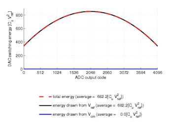
**Figure 3.9:** Energy consumption due to DAC switching for 12-bit ADC using MCS algorithm.
