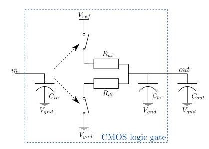
Figure B.1: Conceptual model of one input one output CMOS logical gate.
