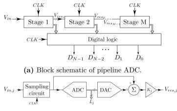
(b) One of stages in pipeline converter.
