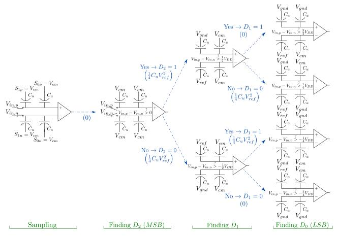
Figure 3.16: 3-bit SAR ADC incorporating asymmetric merged capacitor switching (AMCS) algorithm.
