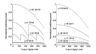
Figure 3.36: Normalized switching power for different distributions of L and M bit values for 10-bit DAC using classical switching algorithm. [32]
