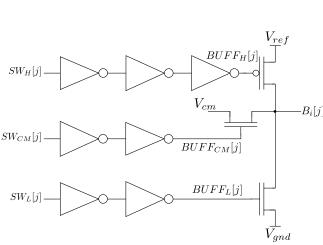
Figure 4.16: Switch with buffers for one of the capacitors of DAC.
