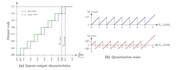
Figure 2.2: Consequences of input signal quantization shown for 3-bit ADC.
