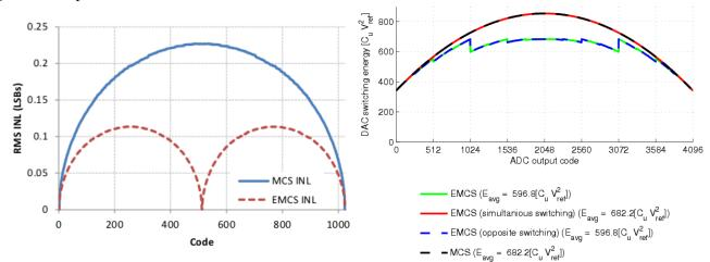
**Figure 3.11:** Comparison of INL for 10-bit ADCs using MCS and EMCS algorithm. [23]
