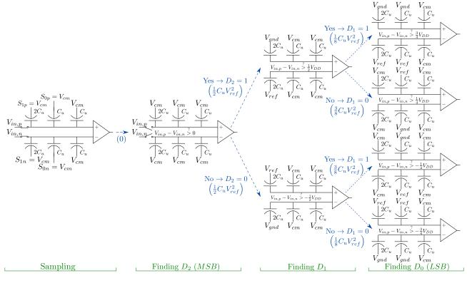
Figure 3.14: 3-bit SAR ADC incorporating early reset merged capacitor switching (EMCS) algorithm.
