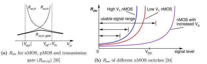
Figure 3.38: On-resistance  $R_{on}$  of transistor switches as a function of input signal level.
