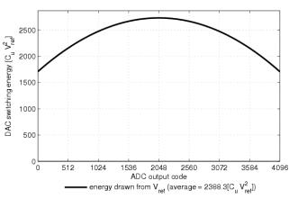
Figure 3.4: Energy consumption due to DAC switching for 12-bit ADC using energy saving algorithm.
