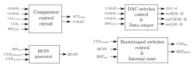
Figure 4.18: Block schematic of designed SAR MCS logic.
