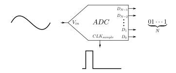
Figure 2.1: Schematic representation of operation of ADC.
