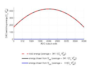
Figure 3.15: Energy consumption due to DAC switching for 12-bit ADC using AMCS algorithm.
