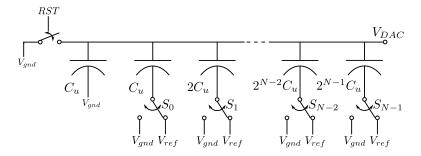
Figure 3.1: Schematic of simple charge scaling DAC.
