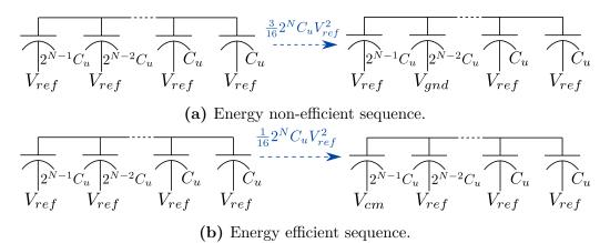
Figure 3.24: Ilustration of idea behind energy-saving switching sequence.
