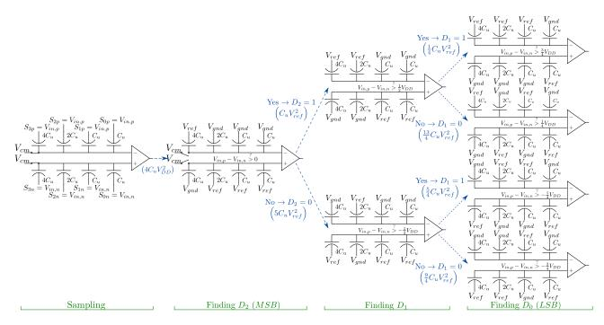
Figure A.1: 3-bit SAR ADC incorporating classical algorithm.
