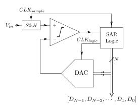
Figure 2.8: Block schematic of simple SAR ADC.
