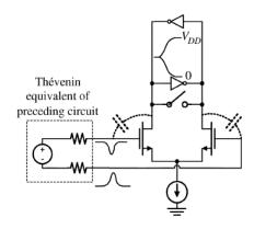
Figure 3.45: Kickback noise generation in latched comparator. [40]
