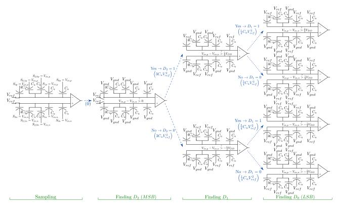
Figure 3.5: 3-bit SAR ADC incorporating energy saving switching algorithm.
