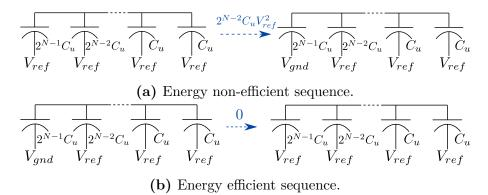
Figure 3.20: Ilustration of idea behind initial switching sequence
