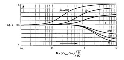
**Figure 3.41:** Charge injection distribution among transistor's source and drain. Reproduced from [34].
