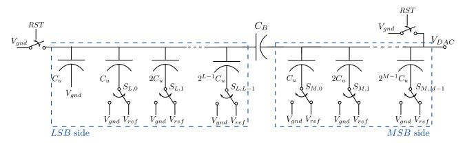
Figure 3.33: Schematic of charge scaling split binary-weighted N-bit DAC.
