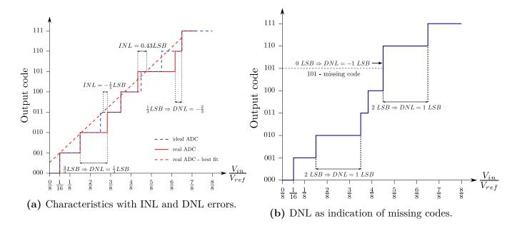
Figure 2.3: Example of INL and DNL errors for 3-bit ADC.
