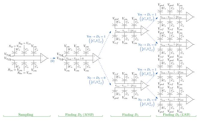
Figure 3.10: 3-bit SAR ADC incorporating merged capacitor switching (MCS) algorithm.
