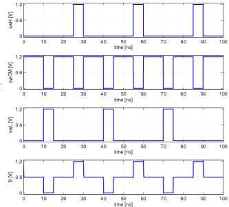
Figure 4.17: Simulated waveform of operations of DAC switch.
