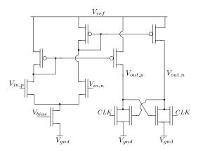
Figure 3.44: Static latched comparator [37]
