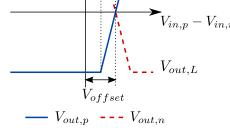
(c) Transfer curve of realistic differential comparator.
