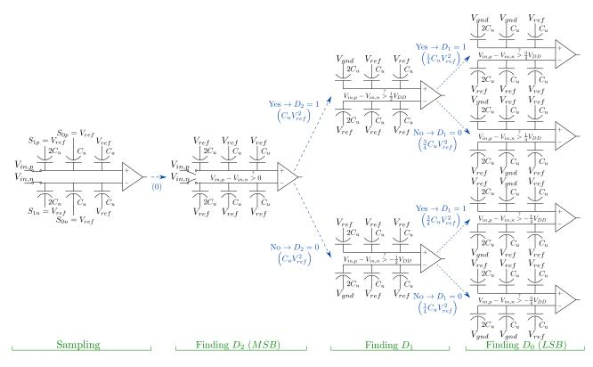
Figure 3.8: 3-bit SAR ADC incorporating monotonic switching algorithm.
