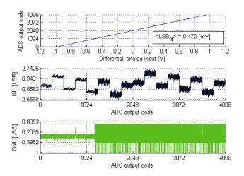
Figure 4.8: Results static simulation (obtained through simulation) for ADCs with MOM-capacitor based DAC extract (rest of the functional blocks – VerilogA).
