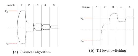
Figure 3.17: Comparison of voltage on DACs top plates during conversion using classical algorithm and tri-level switching. [26]
