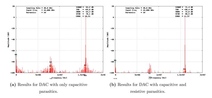
Figure 4.7: ADC performance with MOM-capacitance based DAC (differential input amplitude lowered to 0.88V).
