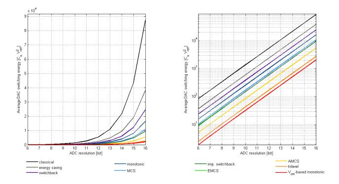
Figure 3.32: Comparison of average DACs' switching energy for different resolutions. For ease of comparison two versions of plot are presented – with linear Y-axis scale (left) and logarithmic Y-axis scale (right).
