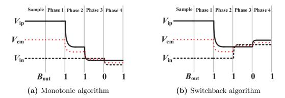
Figure 3.21: Comparison of voltage on DACs top plates during conversion using monotonic and switchback algorithms. [27]
