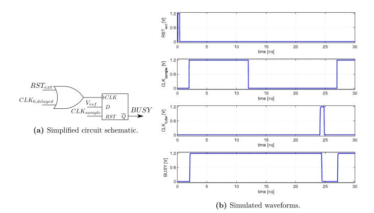
Figure 4.24: BUSY signal generator with simulated waveforms of circuit operations.
