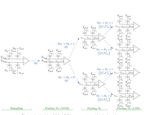
Figure 3.19: 3-bit SAR ADC incorporating tri-level algorithm.
