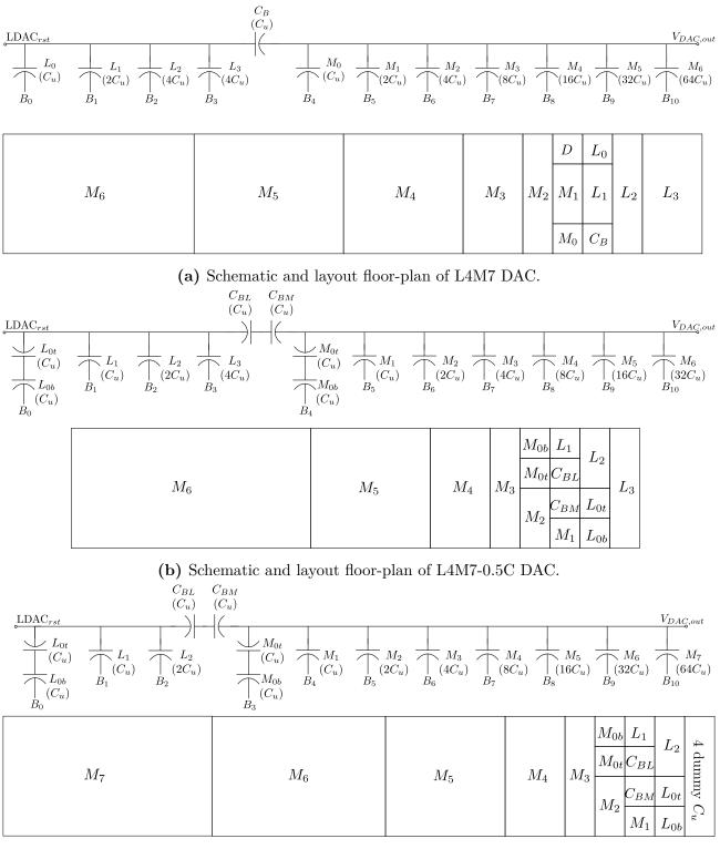
(c) Schematic and layout floor-plan of L3M8-0.5C DAC.
