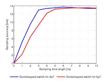
Figure 4.13: Sampling accuracy of designed bootstrapped switches as a function of sampling time.
