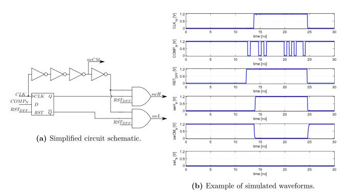
Figure 4.22: Decission circuit schematic together with simulated waveforms.
