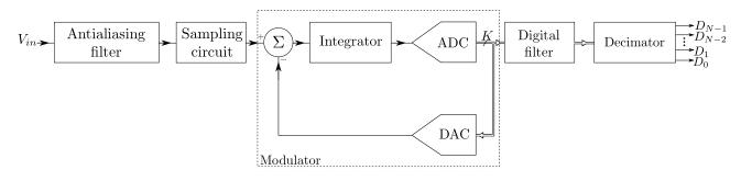
**Figure 2.5:** Block diagram of  $\Sigma - \Delta$  ADC.
