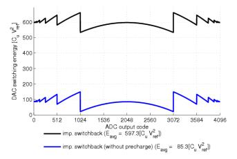
Figure 3.27: Comparison of power consumption due to DAC switching when including and excluding precharge for 12-bit ADC using improved switchback algorithm.
