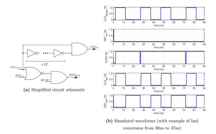
Figure 4.19: Bootstrapped switch control and internal reset generator circuit with simulated waveforms of its operation.
