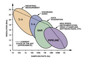
Figure 2.4: General allotment of different architectures of ADC. [17]
