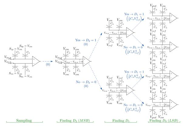
Figure 3.30: 3-bit SAR ADC incorporating  $V_{cm}$  algorithm.
