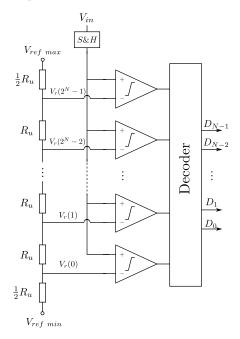
Figure 2.6: Schematic of simple Flash ADC.
